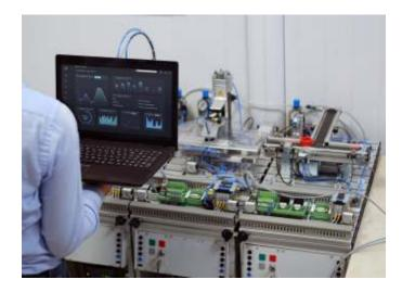
explain how you can add wireless connectivity to PLCs and get bidirectional connectivity for data, reconfiguration, and control, from PLC to your chosen cloud, using Blues Wireless IoT System-on-Modules.
